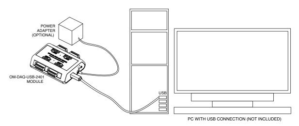
Figure 1-2. System Components
